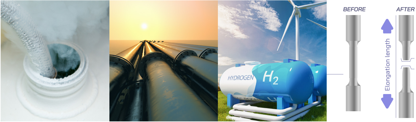
Examples of test specimens that are tested in the lab. Left to right: cryogenic hoses, transport pipelines, (pressurized/cryogenic) storage tanks, small scale material coupon specimens.
