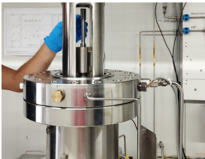
TNO test facility for small scale coupon tests in pressurized hydrogen gas
